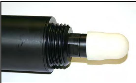
PH electrodes should be stored in such a way to prevent the electrode from drying out. A rubber cap is provided with the electrode for this purpose. A small amount of liquid should be placed in this cap prior to the cap being placed over the electrode. 3M KCl is the preferred storage solution however; tap water should be used if not available. Soaking in pH 4 buffer solution overnight may restore some electrodes that have been allowed to dry out,
