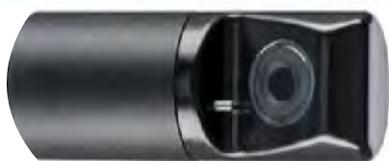
The optical dissolved oxygen (ODO) sensor uses a robust, solid state, fluorescence based transducer for field monitoring in a variety of environments. Fluorescence based sensors are inherently reliable and low maintenance, with no need for replaceable membranes or electrolyte. No Oxygen is consumed during operation making the sensor suitable for low flow applications. The sensor also responds
