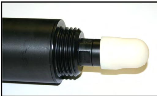
ORP electrodes should be stored in such a way to prevent the electrode from drying out. A rubber cap is provided with the electrode for this purpose. A small amount of liquid should be placed in this cap prior to the cap being placed over the electrode. 3M KCl is the preferred storage solution however; tap water should be used if not available. Soaking in 3M KCl solution overnight may restore some electrodes that have been
