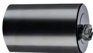
Turbidity is the measurement that indicates the clarity of water due to fine suspended particles. In the environment, turbidity is often due to clay or silt. These fine particles have the ability to scatter light. The MQ/MP Series sensor has a light source that is projected into the water. A detector measures the light that has been scattered at 90 degrees to the source. As the number of particles increase, more light is scattered and sensed by the detector and the higher the turbidity reading.
