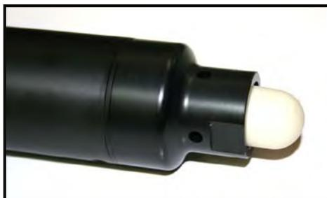
The MQ/MP sensor (with pH or ORP) is shipped with a rubber cap covering the electrode. This cap contains a small amount of 3M KCl solution and is in place to prevent the electrode from drying out during shipping and storage. **This cap must be removed prior to installation.** The cap should be retained so that it can be placed back on the electrode if the sensor is to be removed.
